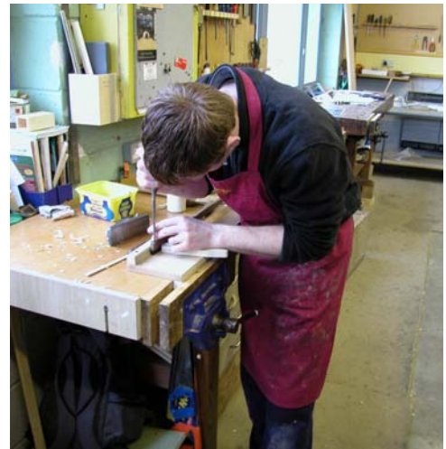
Nick fitting the restored guide pin slot to the keyboard
