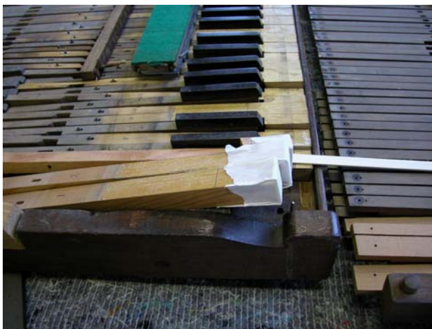
Vertical grained lime glued on the key fronts
