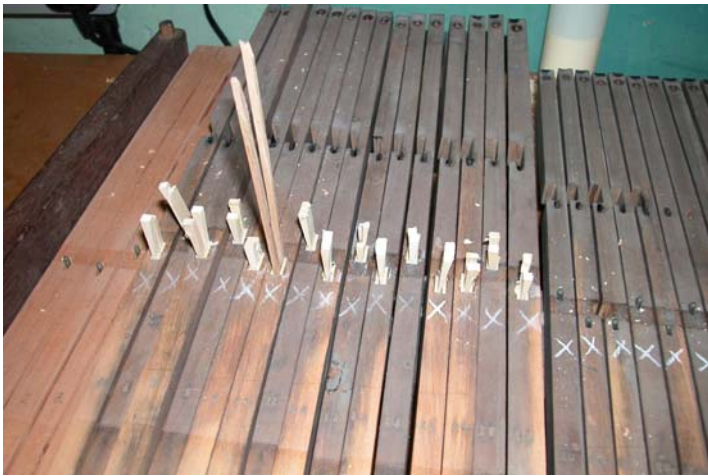
Balance pin slots with new sides glued in
