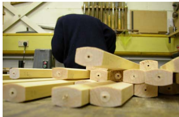
James drilling rollers for the Pedal coupler roller board. The pine rollers have an insert of lime for better wear.
